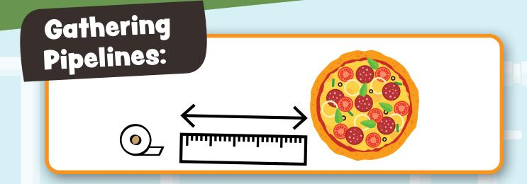
Gathering pipelines carry oil and gas from the wells (where these products are pulled out of the ground) to the facilities where they are processed (made into fuel we can use). These pipes stretch across 250,000 km and have openings anywhere from the size of a roll of paper towel (101 mm) to the size of a large pizza (304 mm).<sup>14</sup>
