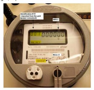
• When the identification number on the left of the screen is 46, the main number displayed will be imported kWh to the grid, so the power the customer is exporting to the grid
