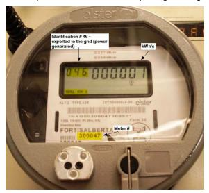
When the identification number is 888, this is a segment check test
