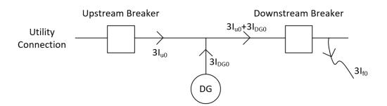
The de-sensitization of concern is the fault flow currents designated  $3l_{u0}$  in the diagram above.
